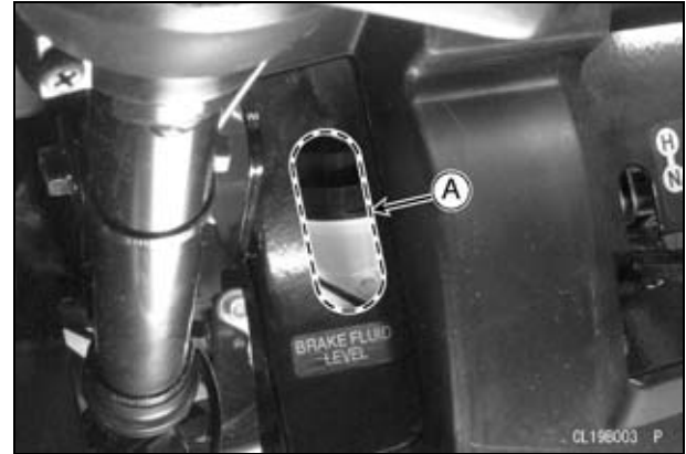
A. Inspection Hole
