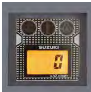
Tachometer with warning indicators
